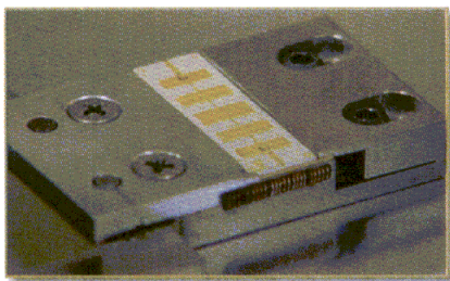
Fig. 3 The test/tune fixture of the tuning station has two positions on a precision slide for either testing or tuning.
